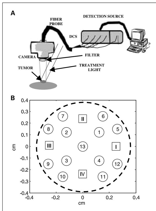
**Fig. 1.** A schematic of the DCS instrument (A) and a map (B) of the probe for measuring tumor blood flow. Optical fibers for 13 source positions (small circles) and four DCS detectors (squares) are arranged in a two-dimensional pattern. Large dashed circle, contour of the tumor.
